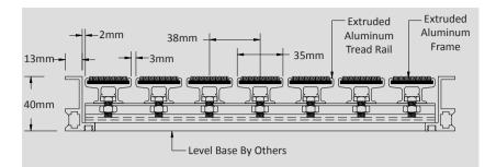
• Maximum dimensions(1 unit): 6 metres wide, and without limits in the walking direction.
